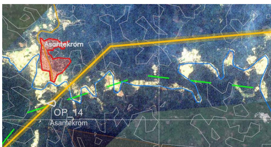
Figure 18: Satellite image showing the optimised crossing of the River Disue and the practice of galamsey along the river The route crosses the Asankragua-Enchi road twice and then the Tano (or Tanoé) river.
